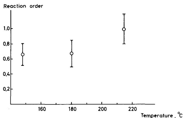
FIG. 1. Reaction order with respect to hydrogen in methyl linoleate hydrogenation in vapor phase at different temperatures. The confidence limits are at the 95% level.
